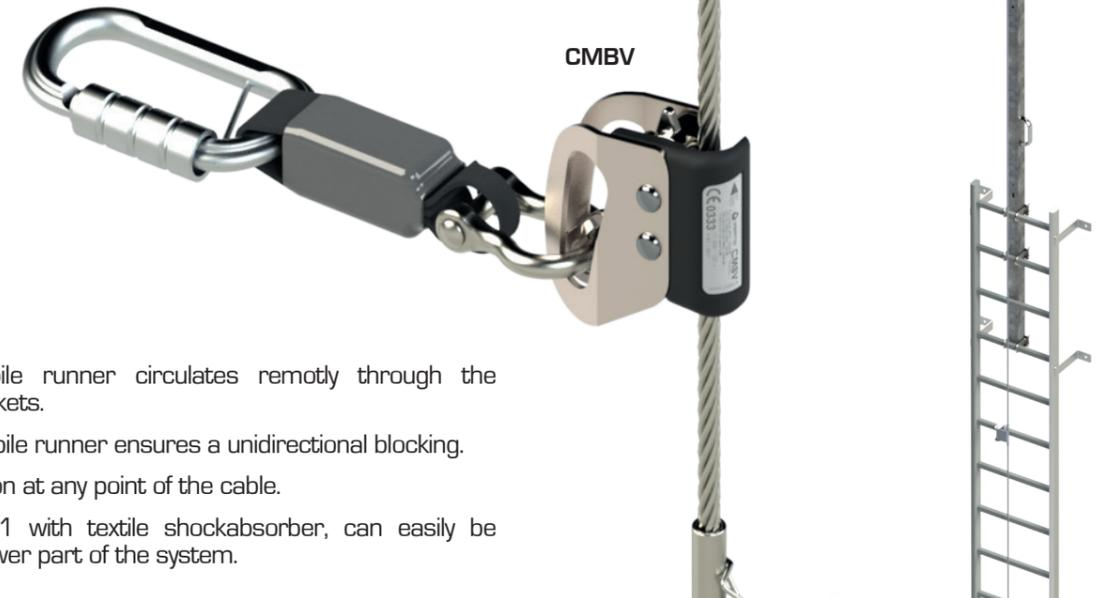
The CMBV mobile runner circulates remotely through the intermediate brackets.
